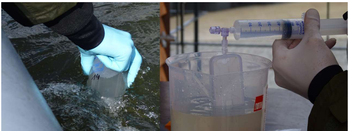
Figure 11 Sampling steps of eDNA sampling. Left: Taking water subsample for mixed samples. Right: Filtering eDNA from mixed sample.
